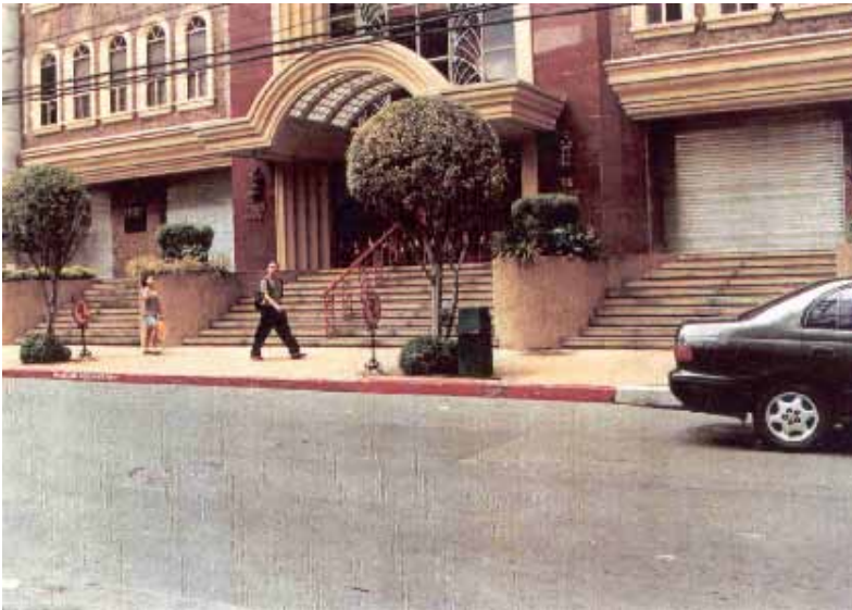
Illustration 11 10 steps with no ramp, leading to the main entrance of a residential condominium.
