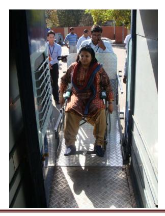
3. Person with reduced mobility, used an aisle chair with castors (provided by Callidai) and could also successfully embark, reach upto the berth in the aisle chair and disembark the standard coach through the Mobile lift.
