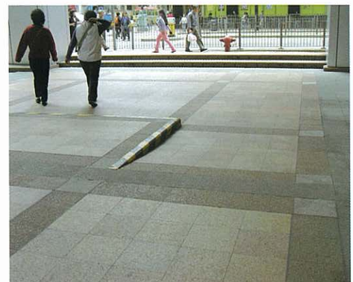
Fig 1. Avoid unexpected steps and levels.
