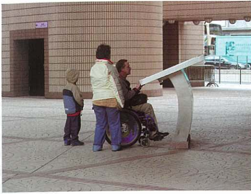
Fig 6. Provide accessible way finding information to different users. The addition of a tactile map or audible system facilitates access by people with visual impairment.
